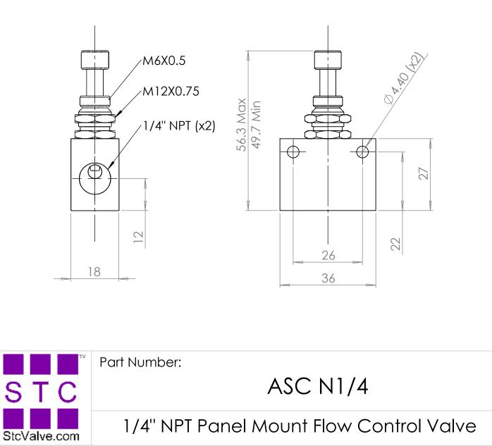
Information in the drawing is provided for reference only. Dimensions are in mm, U.N.O.
