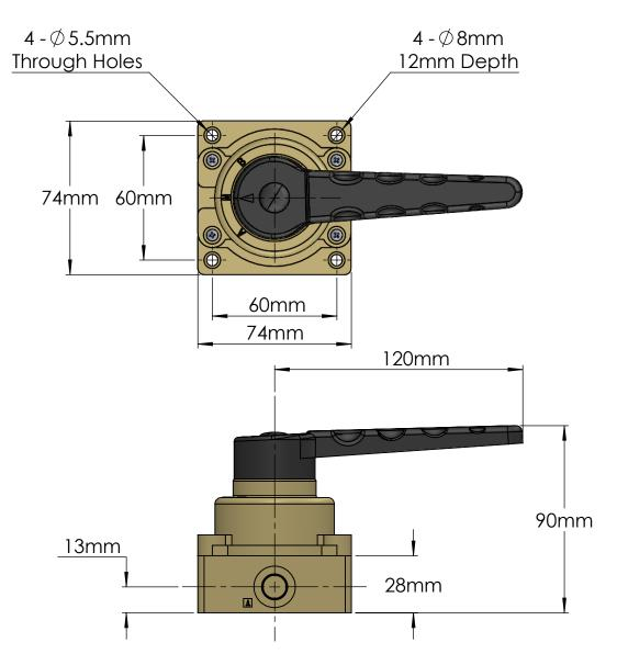
\*NOTE: HV 410 = 2-Position, HV 420 = 3-Position, Closed Center
