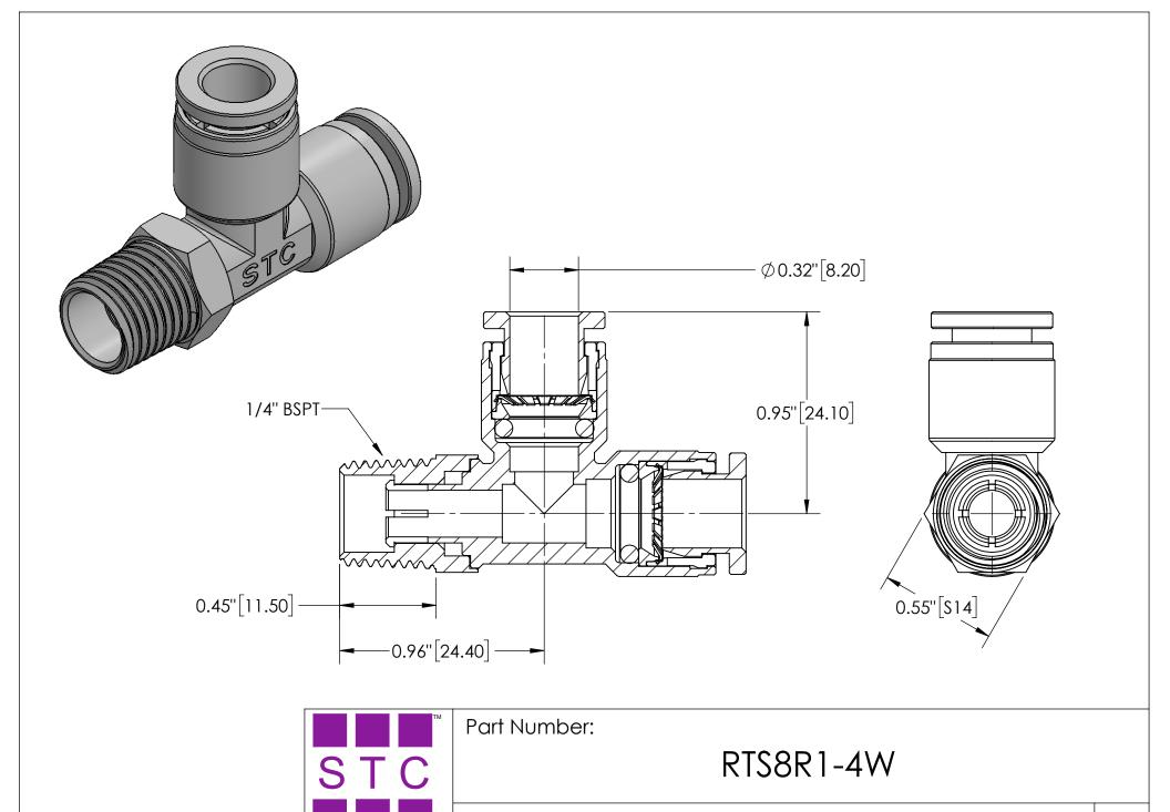
316 Stainless Steel Run Tee (Swivel), 8mm Tube, 1/4" BSPT Thread
