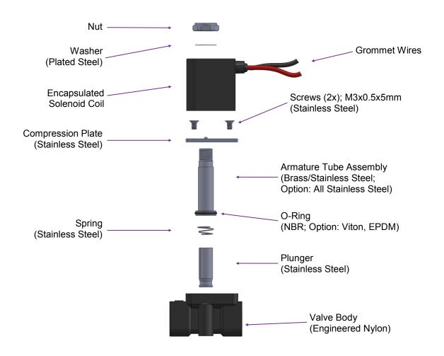
**Note:** Standard configuration is shipped with a DIN coil (as shown in the title page picture, as well as in the diagram on page 6). Grommet coil (above) is available by request.
