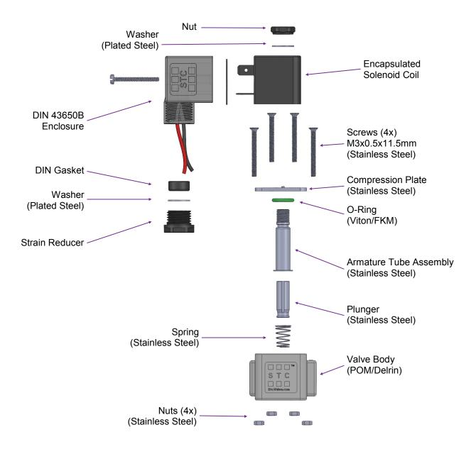
**Note:** Standard configuration is shipped with a DIN coil (as shown above). Grommet coil (lead wires) is available by request.
