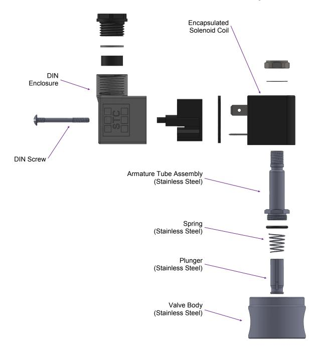
Note: Standard configuration is shipped with a DIN coil (as shown above). Grommet coil is available by request.
