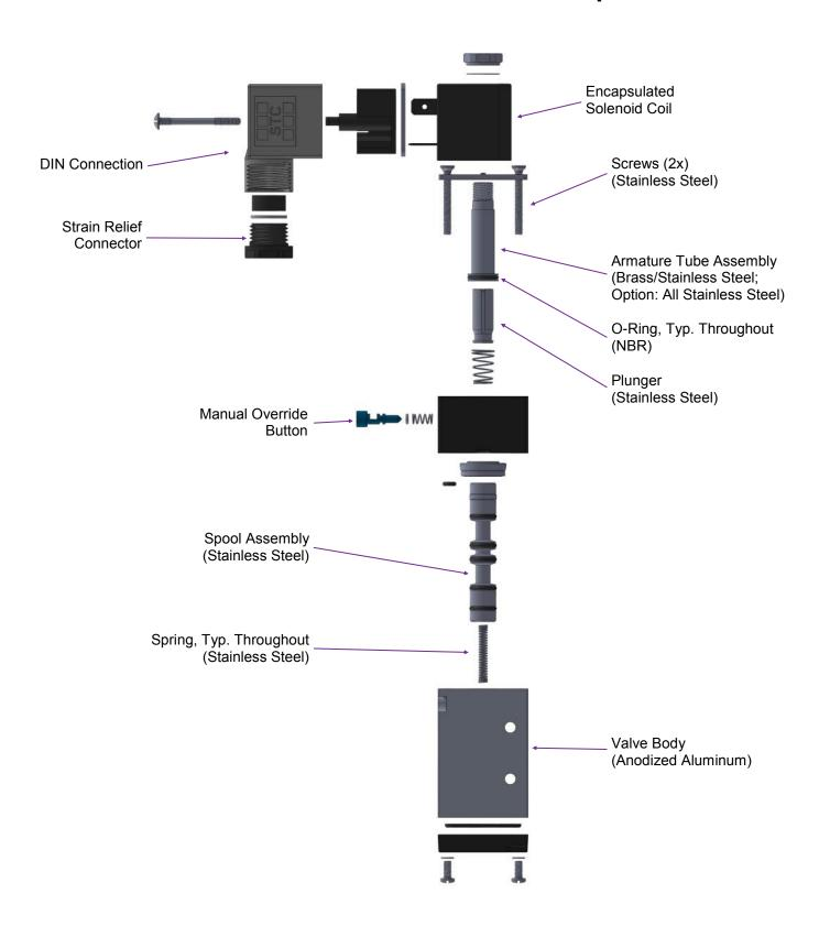
**Note:** Standard configuration is shipped with a DIN coil (as shown above). Grommet coil (lead wires) is available by request.
