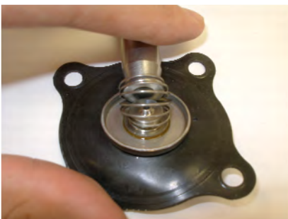
Figure 6: Diaphragm. Debris in the center hole may cause valve malfunction
