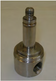
Figure 1: Complete assembly of the direct acting valve.
