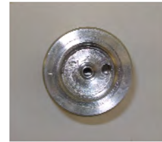
Figure 3: Valve body. Debris around the center hole may lead to valve malfunction.
