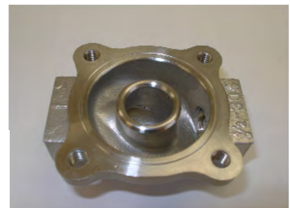
Figure 7: Lower body. Debris in the lip of the inner chamber may cause valve malfunction
