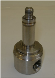
Figure 1: Complete assembly of the direct acting valve.
